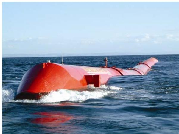
**Fig 1. The prototype PELAMIS (photo courtesy OPD Ltd., Edinburgh, UK)**
